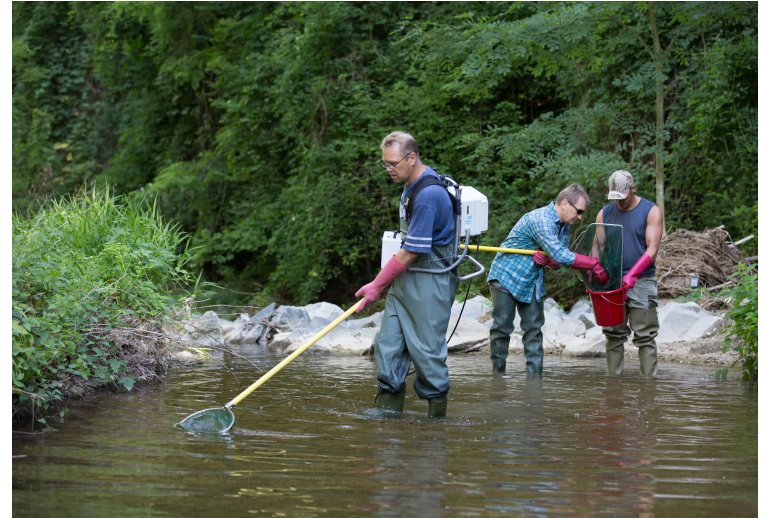
An illustration of backpack electrofisher Source: NMK - Ichthyology
